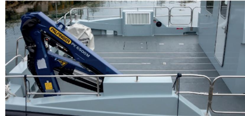
The spacious, flat after deck with optional crane allows for a wide range of payloads to be embarked or tasks to be conducted safely, and with ease. The deck features a deck rail system, common with the rest of the SEA Class range, to provide easy and rapid restraint of any deck cargo.
