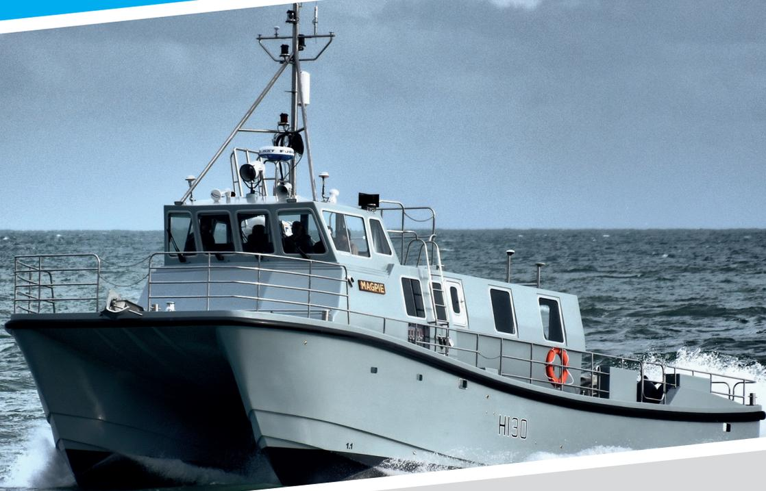
The 18m SEA Class Survey Motor Launch is the largest variant of the SEA Class range. Renowned for its sea keeping capability, the craft offers AEUK's modular and fully integrated capability for hydrographic survey. The craft is equipped with Single and Multi-beam Echo Sounders, motion reference equipment, as well as the S2094 towed side scan sonar system.
