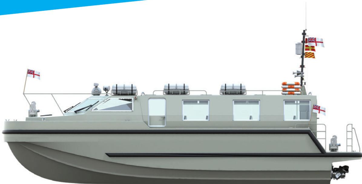
The Passenger Transport variant of the SEA Class range of workboats is a ship-launched craft. It is equipped with industry leading Whole Body Vibration (WBV) isolation seating for up to 36 passengers.
